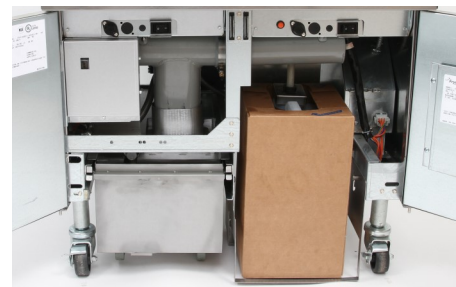
Figure 1: The fryer prior to the install is show above. The sensor mounts on the channel behind the center upright. The pre-filter mounts above the filter pan pickup .
