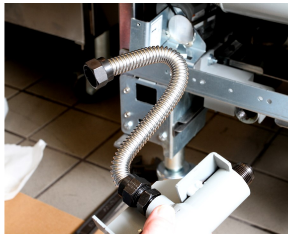
Figure 3 : Shape the flexline attached to the pre-filter to route to the filter pan pickup.
